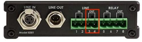
2. Once connected, dial the Algo 8301 extension's number from an account phone. A tone will play, confirming connection to the Algo 8301, and a second dial tone from the analog paging system will start. Enter your analog dialing/paging codes to use the analog system.
