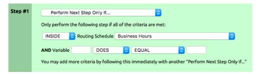
Once a call reaches this extension, the system will check to see if the call is INSIDE the routing schedule called Business Hours. If the call is inside the hours specified, then the call will progress to step 2. If the call is outside the scheduled time, it will skip step 2 and proceed to step 3.
