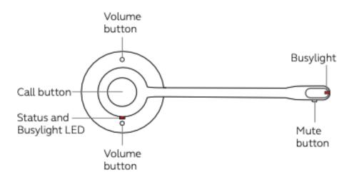
Power on: Press the call button on the headset or undock the headset from the base
